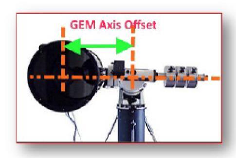
Again, this is a tricky one because it's in the middle of a solid object. This may be best approached by measuring from the intersection point to the top of the saddle plate, then from the saddle plate to the centre of the telescope tube (or, measure the diameter of the tube and divide by 2 to get radius). Then add those two together:
