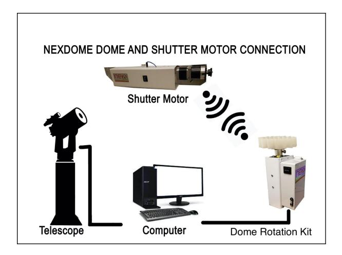
**Dome Rotation Unit (with and without rain sensor versions)**: This unit is the main controlling unit that is connected to the observatory computer and rotates the dome in azimuth. The dome rotation unit also communicates with the (optional) Dome Shutter motor unit.
