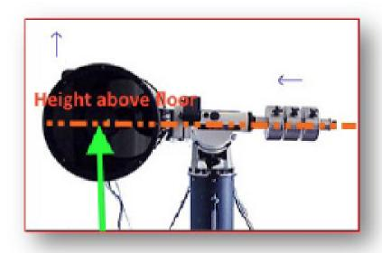
Then subtract the height of the dome rim (1350 mm from the schematic drawings) to give your up/down offset.
