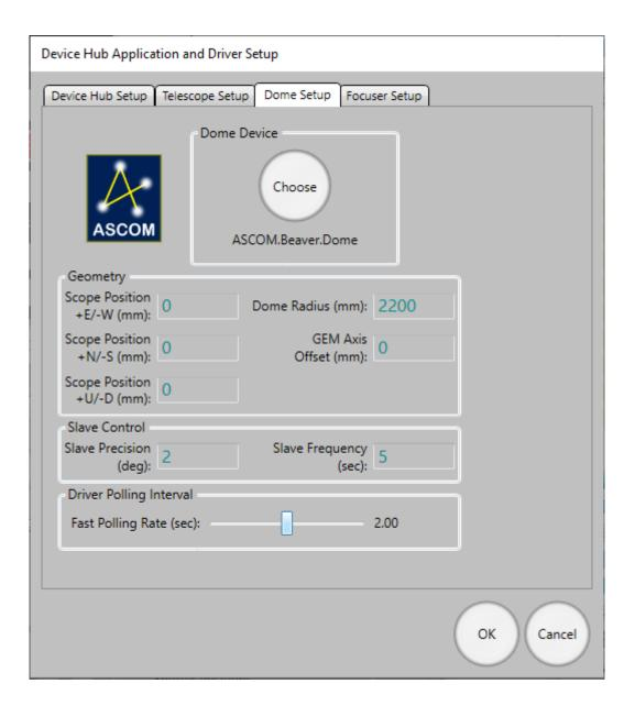
The computations required for scope-dome synchronization are nontrivial and somewhat sensitive to small input errors. Therefore, to get accurate scope-dome synchronization across the whole sky, your geometry settings must be as accurate and precise as possible.
