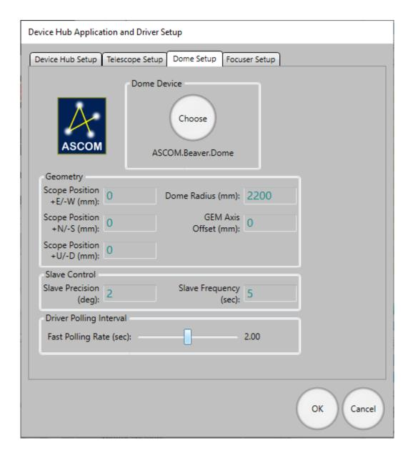
Unless our telescope rotation center is perfectly centered on the dome, and using a fork mount, we need the software to correct for that misalignment of the axis.
